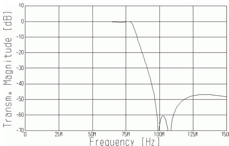
**Figure 2: Low-pass filter LPF[6] simulated transfer**
