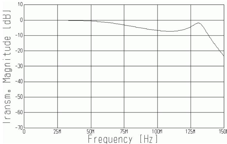
**Figure 5: PA output filter simulated transfer**
