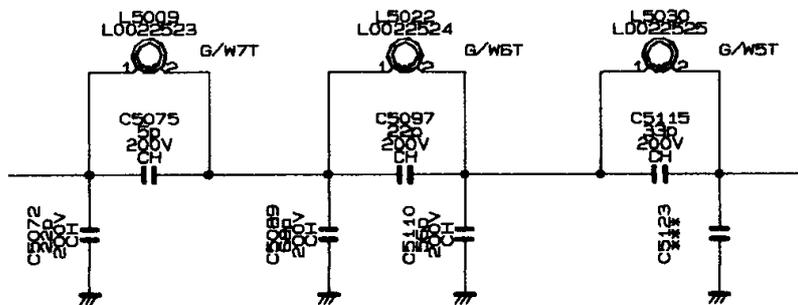
Figure 1: Low-pass filter LPF[6] circuit diagram
