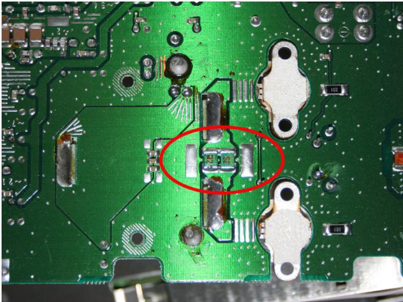
**Figure 8: Unmodified PA output**
