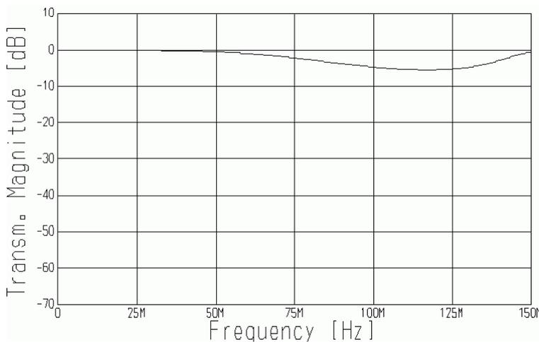
**Figure 6: PA output filter without C5058 simulated transfer**
