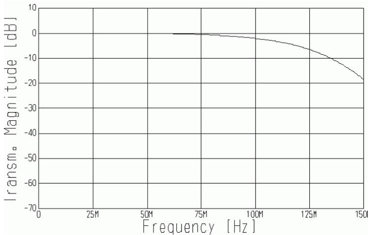
**Figure 7: PA output filter without C5050 and C5051.**
