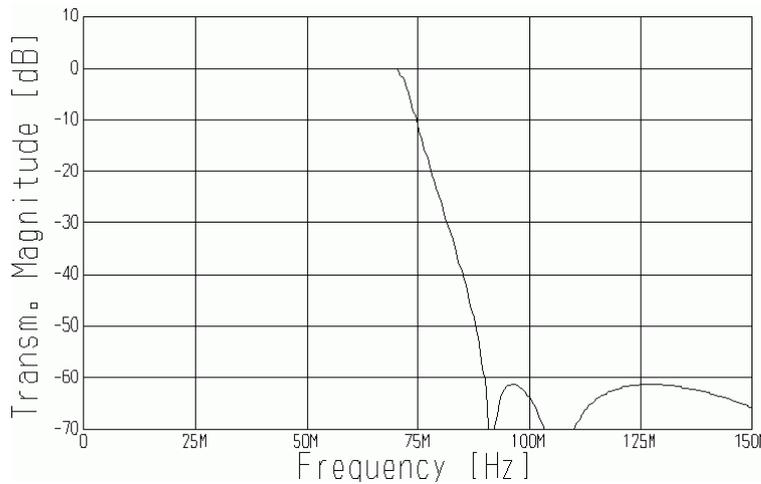
**Figure 3: Low-pass filter LPF[6] without C5123 simulated transfer**
