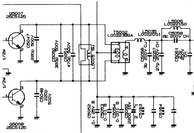
**Figure 4: PA output filter circuit diagram**
