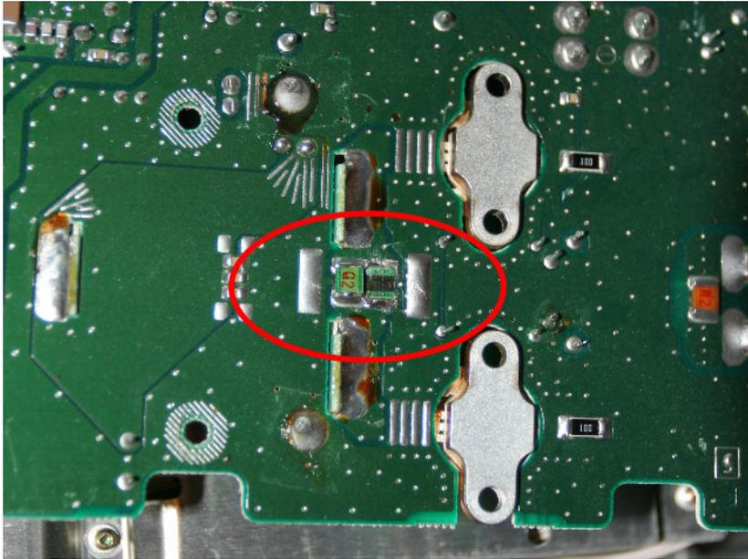
**Figure 9: PA output without C5051**
