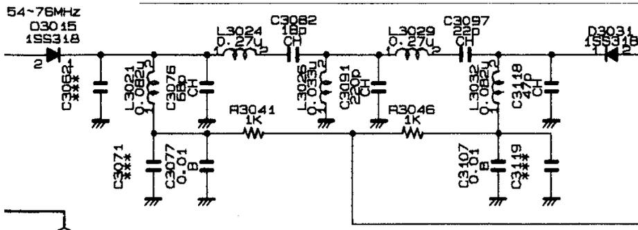
Figure 3: “Original Yaesu FT-847 54-76 MHz TX filter” circuit diagram
