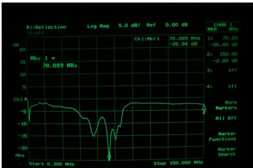
Figure 13: Transceiver input reflection measurement for 54-76 MHz band.
