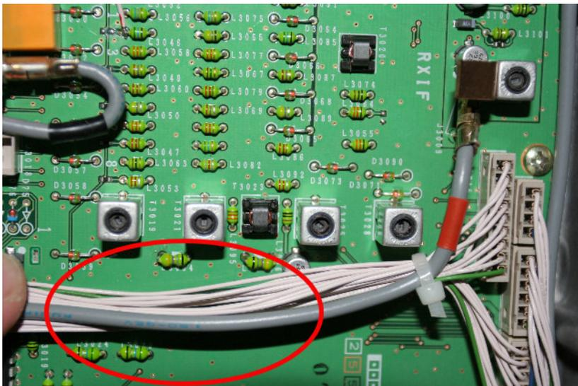
**Figure 11: PCB top view of the modified 54-76 MHz RX and TX filters**
