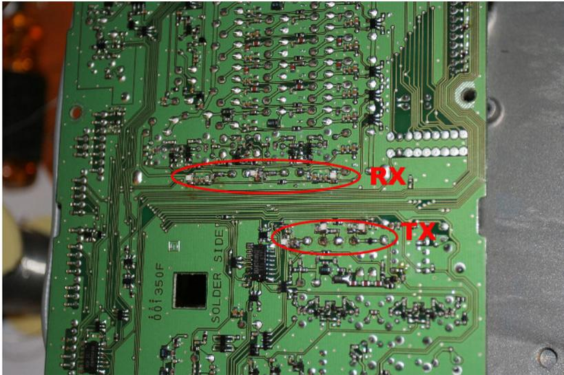
Figure 12: PCB bottom view of the modified 54-76 MHz RX and TX filters
