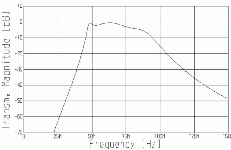
Figure 4: “Original Yaesu FT-847 54-76 MHz TX filter” simulated transfer
