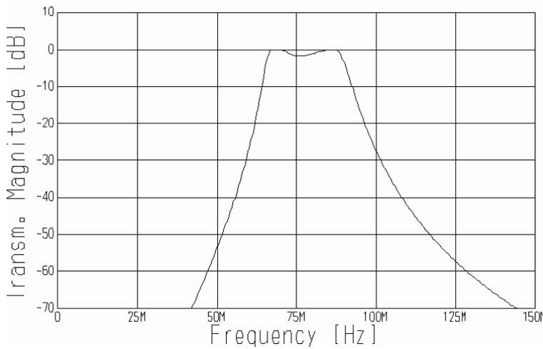
**Figure 10: “UK factory mod 70 MHz TX filter with correct inductor values” simulated transfer**
