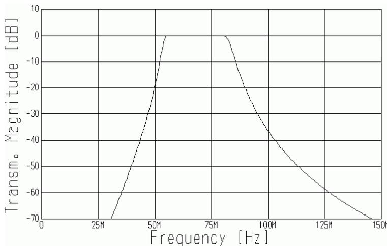
**Figure 8: “PA10 54-76 MHz RX filter” simulated transfer**
