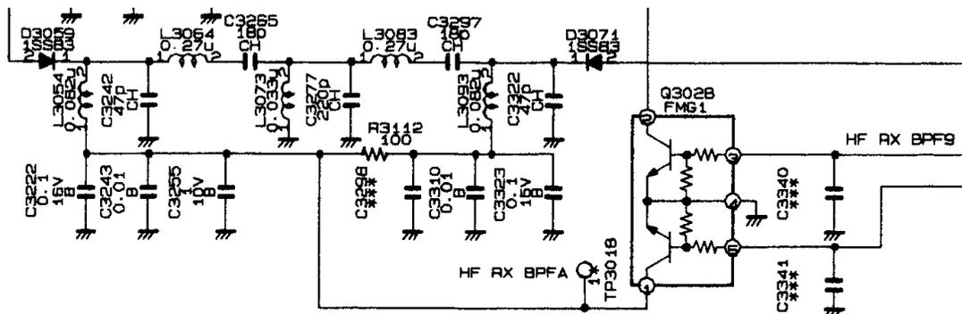
Figure 1: “Original Yaesu FT-847 54-76 MHz RX filter” circuit diagram
