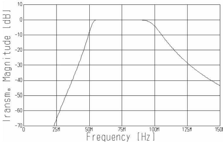
**Figure 7: “Might have been Yaesu FT-847 54-76 MHz RX filter” simulated transfer**
