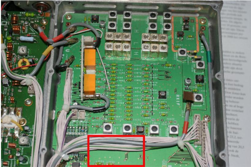
**Figure 5: PCB top view of the original 54-76 MHz RX and TX filters**
