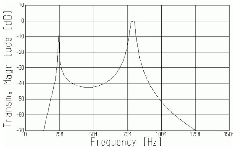
**Figure 9: “UK factory mod 70 MHz TX filter on the internet” simulated transfer**
