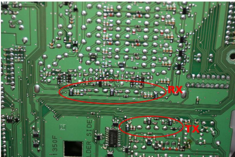
**Figure 6: PCB bottom view of the original 54-76 MHz RX and TX filters**
