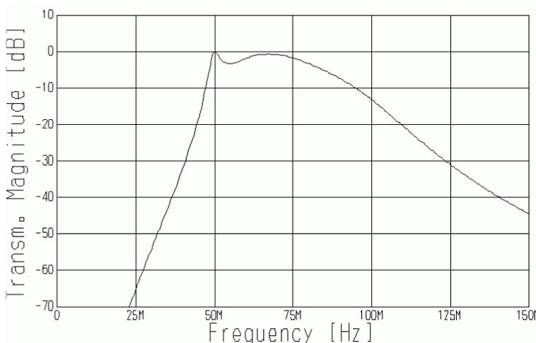
Figure 2: “Original Yaesu FT-847 54-76 MHz RX filter” simulated transfer
